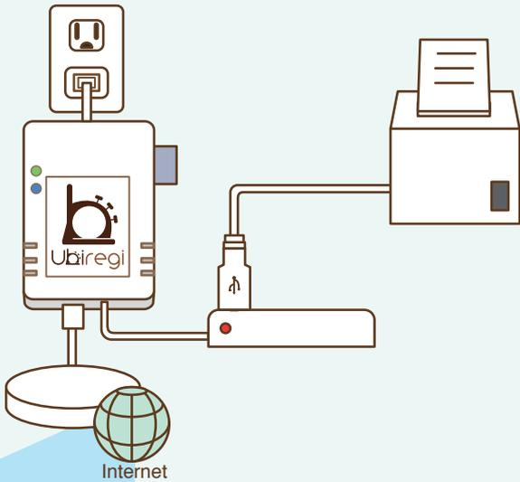
1. Put the SD card into the Extension and connect it to the USB hub and Ethernet cable. Plug the electrical cord into the outlet. Check to make sure the Extension lights are lit up.
